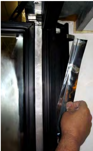
Step 3: Remove reflector plate.
